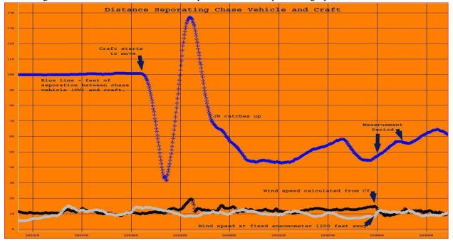
DDW 13) The primary off board wind direction and velocity measurement instruments were on the chase vehicle. As seen on the blue line above, the chase vehicle briefly got about 140 feet away as JB ran back to the chase vehicle after push starting it. During the measurement period he was 48-57 feet away. Note: there was also good agreement between the chase vehicle true wind values and a fixed anemometer (1200 feet away). This reflects the relatively steady wind speed when this run was made.
